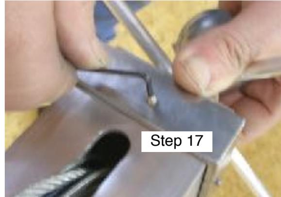
the nut. Tighten the nut. Get your other bracket, align the two outer holes of the winch bracket to the winch, insert bolts from the inside of the winch, and tighten nuts using your 1/2" wrench. (See photos Step 18A, B, and C). You want your brackets to have the open side face towards the ground as seen in the photo 18D on page 6.
